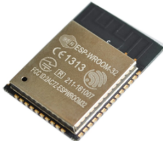
ESP32 module: ESP-WROOM-32
